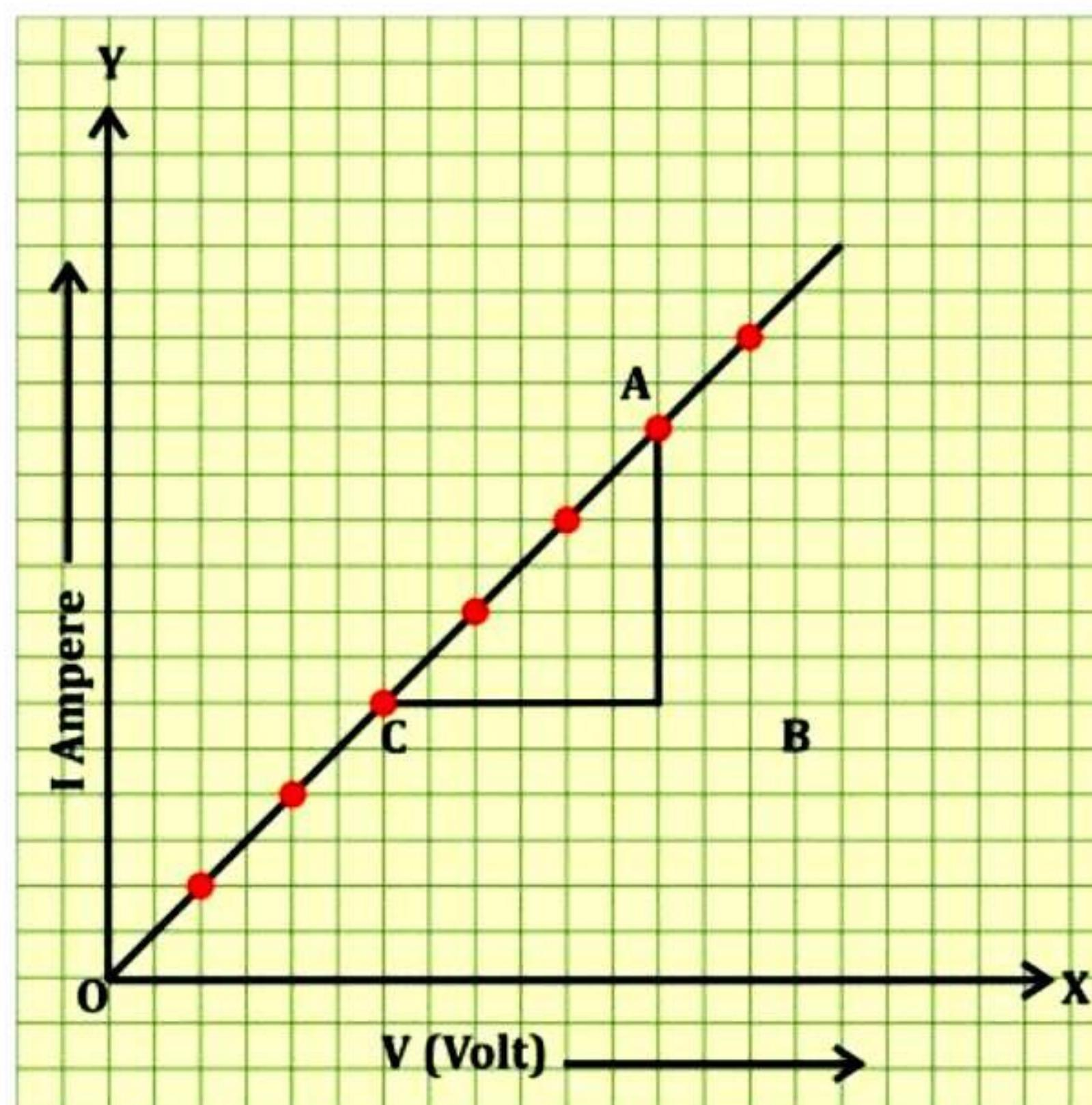
Resistance of wire two from the graph,  $R = \frac{BC}{AB}$  (i.e. reciprocal of slope of the graph)  $\approx 4\Omega$
