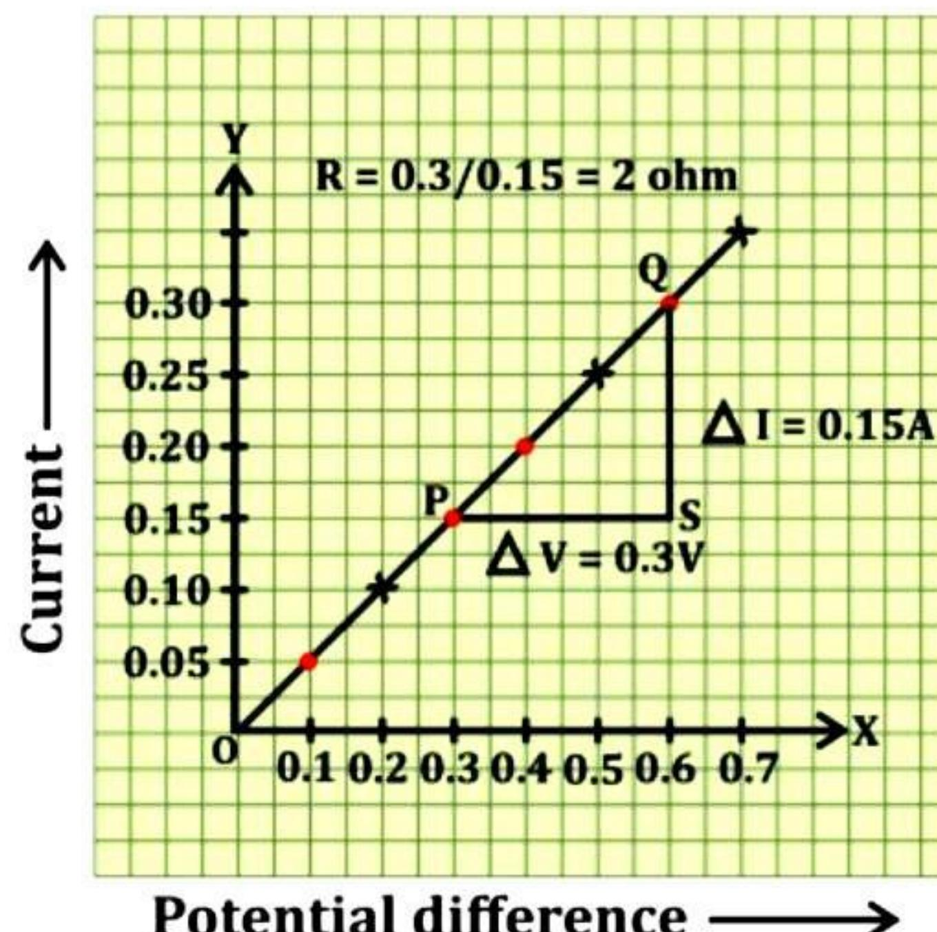
Resistance of wire one from the graph,  $R = \frac{PS}{QS}$  (i.e. reciprocal of slope of the graph)  $\approx 2\Omega$
